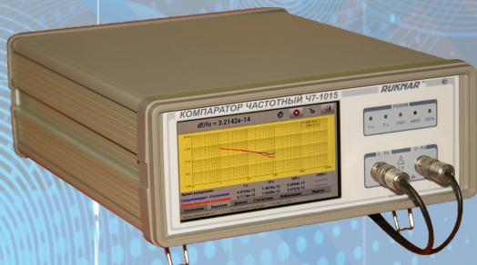
Frequency comparator CH7-1015 is intended for use as a simple and precise instrument for measurements of the relative frequency difference of precision crystal oscillators and rubidium frequency standards, calculation of metrological characteristics (Allan and Hadamard variances, standard deviation, drift, median value etc.) with the mapping process and the measurement results on the internal display or an external PC. PC software included. Remote desktop and remote control are supported.
