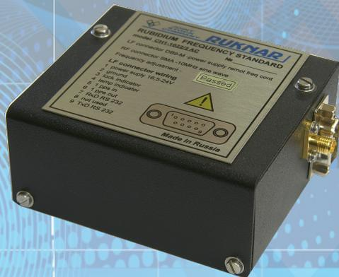
A compact CH1-1022/3 rubidium frequency standard is intended for use as an embedded signal source for frequency and time measuring systems, telecommunication systems and navigation. Rubidium clock with user-programmable output signal frequency as well as digital control and monitoring via RS-232 port. The device is designed for applications with high demands on the size, weight and power consumption. Available options: B - improved short-term stability. PC software included.
