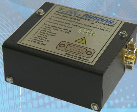
A compact CH1-1022/2 rubidium frequency standard is intended for use as an embedded signal source for frequency and time measuring systems, telecommunication systems and navigation. Disciplined by external 1pps signal rubidium clock with digital control and monitoring via RS-232 port. The device is designed for applications with high demands on the size, weight and power consumption. Available options: B - improved short-term stability; C - improved
