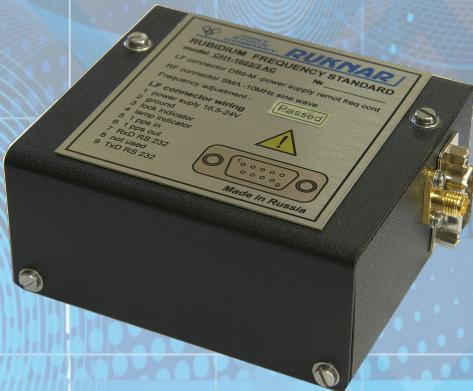
A compact CH1-1022/1 rubidium frequency standard is intended for use as an embedded signal source for frequency and time measuring systems, telecommunication systems and navigation. The device is designed for applications with high demands on the size, weight and power consumption. Available options: B - improved short-term stability; C - improved phase noise; D- fine frequency tuning (step  $1 \cdot 10^{-14}$ ). PC software included.
