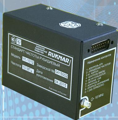
Small CH1-1012 rubidium frequency standard is intended for use as an embedded signal source for high stability frequency and time measuring systems, telecommunications systems and navigation. The device is designed for mobile applications with high demands on the size, weight and power consumption.
