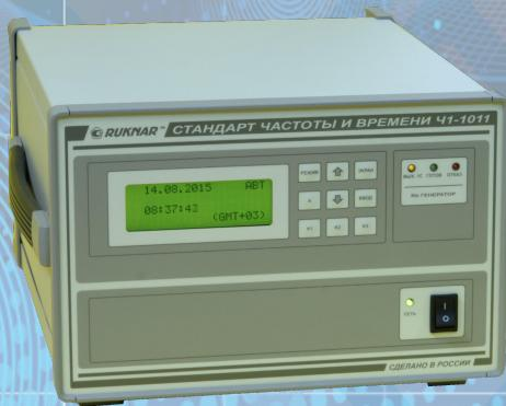
Rubidium time and frequency standard CH1-1011 is intended for use as a high stable source of signals with frequencies of 1, 5 and 10 MHz in various frequency & time measuring systems. It features high frequency stability and spectral purity of the output signals. GPS/GLONASS disciplined rubidium standard. Synchronized by GPS/GLONASS or external time scale 1pps output. All-digital
